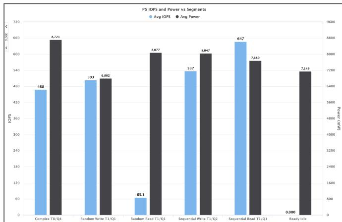
**Test Reports.** Required test results are automatically generated in Excel and html formats. Above shows workloads, IOPS and Power.
