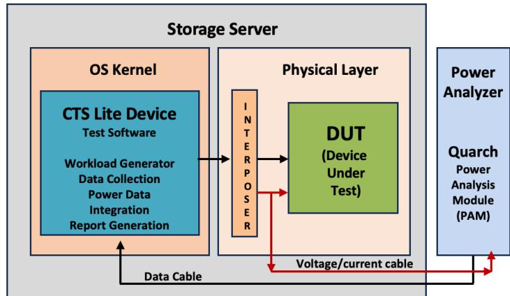
CTS Lite Device benchmark testing for individual storage device level power efficiency measurement shown with Quarch Device Power Analysis Module.
