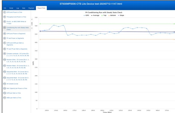
**SNIA 5-Round Steady State Determination.** CTS Lite Device automatically generates results plots (P1-P17). Plot P4 above shows Conditioning run with Steady State Check.
